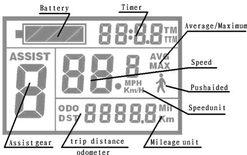
battery indicator, trip time(TM), motor power ratio(ASSIST), current speed,trip distance (DST), 6Km/h assistant power mode, electrical system malfunction code.
